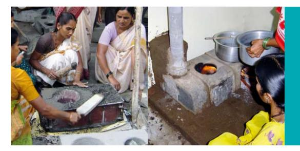
Made from clay and concrete, the stoves are simple to use and maintain. Unlike conventional chimneys, the Chulha stove has a chimney assembled from several sections, making it easier to manufacture and transport. It can also be opened up and even partly disassembled for cleaning.
